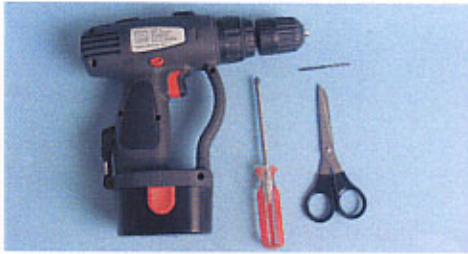
1. Fitting tools required include star point screwdriver, scissors, drill & Ø2.5mm drill bit
