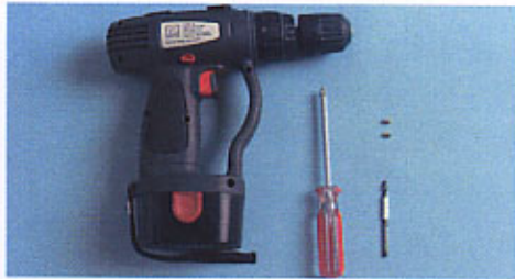
a1. Fitting tools required include Ø4mm drill bit and star point screwdriver
